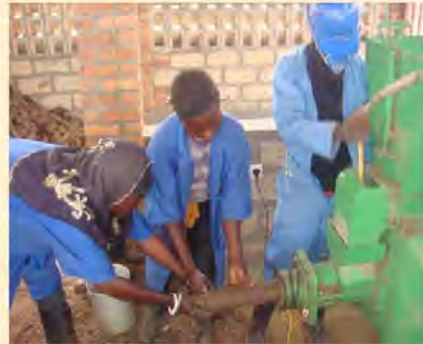
DIF-purchased machine that transforms household organic wastes into household energy by making clean-burning briquettes from the recycled wastes
